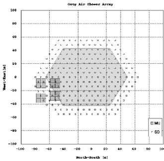
Figure 1: The GRAPES-3 experimental system with 257 scintillator detectors and 16 muon detector modules
