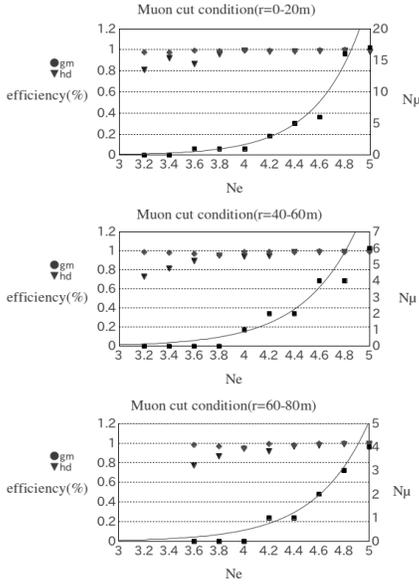
Figure 4: Muon cut conditions for several shower size and area in the GRAPES-3 air shower array. Circle shows the gamma ray detection efficiency and triangle shows the proton rejection efficiency.
