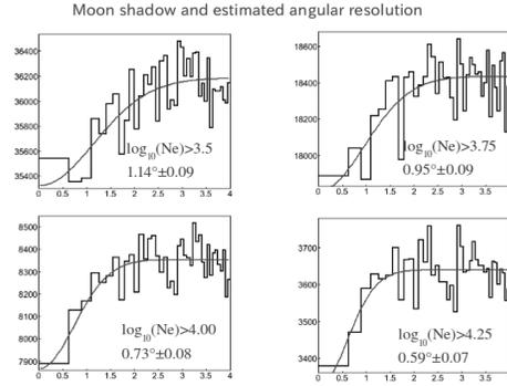
Figure 5: Moon shadow seen in various annular regions centered on the direction of the Moon for four energy regions, with the data period from 2000 to 2006.
