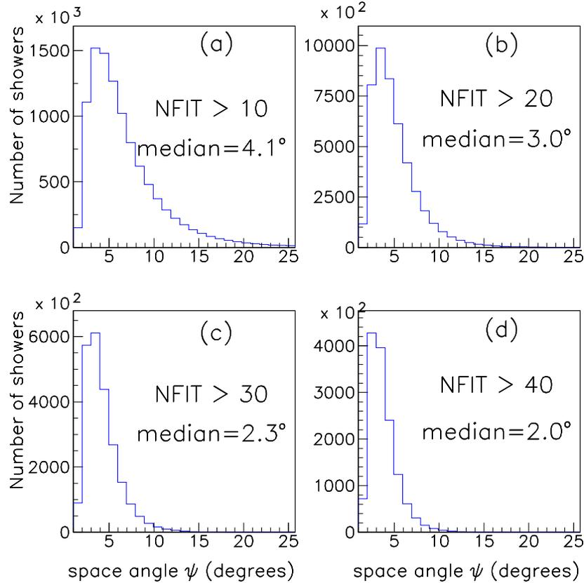
**Figure 5.** space angle distribution between Even and Odd array as a function of number detectors participated in the angle fit (NFIT). The width of the distributions become narrower from (a) to (d) which tells that the angular resolution is better with more number of detectors.
