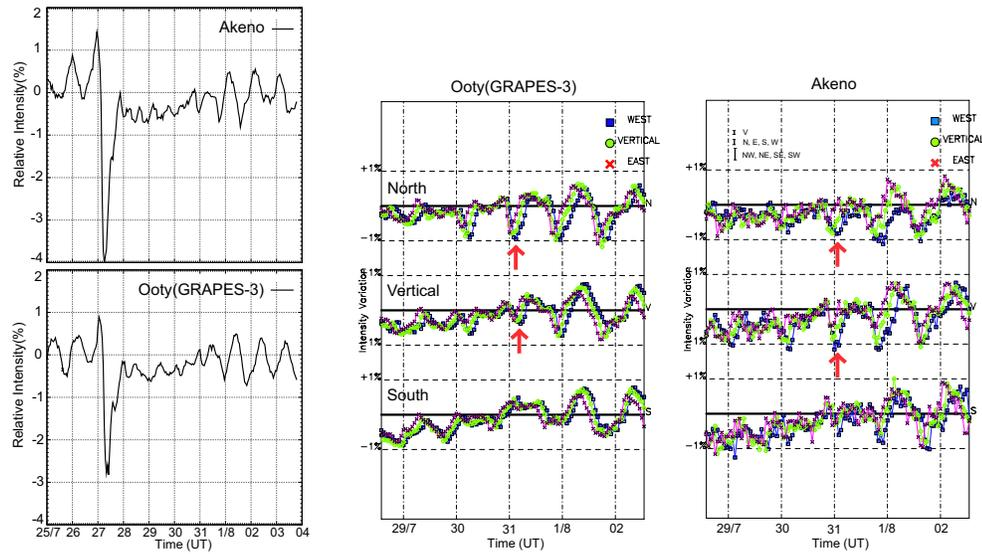
**Figure 3.** Relative muon intensity at Akeno and Grapes-3 muon telescopes. Left: Variation in muon rate observed at GRAPES-3 and Akeno are shown. Statistical errors in GRAPES and Akeno are 0.036% and 0.01% respectively. Center: Variation in 9 direction at GRAPES-3 are shown. Statistical error for each series is 0.09% to 0.15%. Right: Variation in 9 direction at Akeno are shown. Statistical error for each series is 0.018% to 0.029%.
