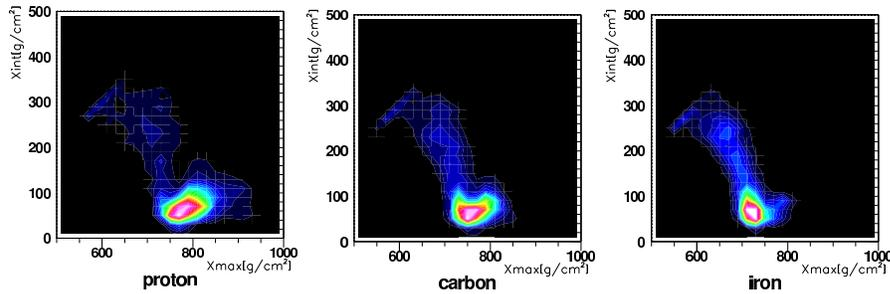
**Figure 1.** Two dimensional distributions of  $X_{\text{int}}$  and  $X_{\max}$  for reconstructed events which are simulated of primary protons(*left*), carbon nuclei(*center*), and iron nuclei(*right*).
