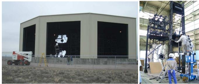
**Figure 2.** The left panel is an external view of the fluorescence detector station. In this picture the shutter is open, and then a telescope mount held segment mirrors is seen. The right panel is a close-up view of a telescope mount. The lower part of it held segment mirrors and an imaging camera. The picture was taken at a workshop of a production company in Japan.
