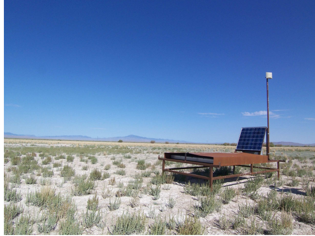
Figure 3.37: The surface detector deployed TA site.
