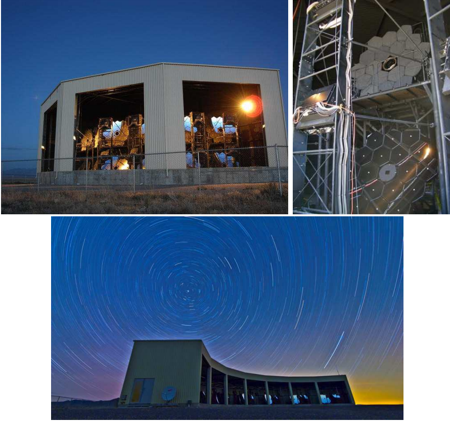
Figure 3.2: The BRM station (top-left), the florescence detectors of BRM station (top-right) and the MD station and MD fluorescence detectors transported from HiRes-I and HiRes II experiment (down).
